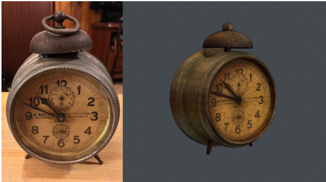
Photo 7. On the right the clock designed for scanning, on the left the model obtained in the scanning process (my own source)
